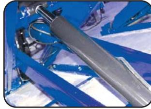
Quad-counterpoised lifting system and 4 powerful heavy-duty cylinders maintain a constant level from floor to full lift height.
