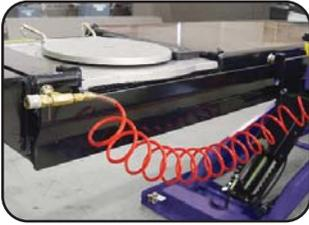
A port can be added in for customer supplied quick disconnect allowing for an easy air tool connection point.
