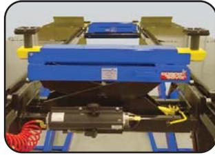
Roller Jacks incorporate a low-profile design - eliminating the need to swing away when the lift is lowered. High lifting heights enable more access for undercar repairs.
