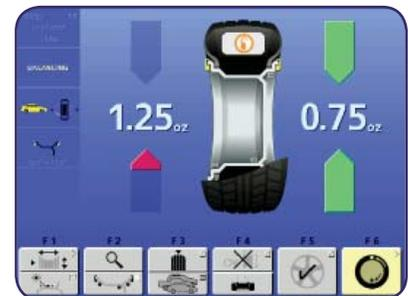
The inner scanner determines the wheel edge profile for the weight type as defined by industry recognized standards for clip weight type. The clip shape and weight color code is indicated across the top row of the weight usage chart. Weight amounts are listed along the side. Upon un-clamping the wheel, the weight type, including both clip type and adhesive weight type, and weight amount are written to the Weight Wizard weight usage tracking file.
