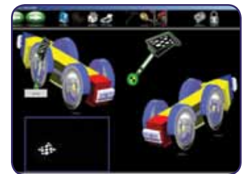
Live camera view aids technician in target placement.
